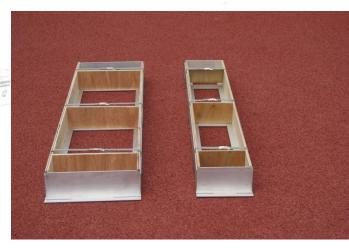
Foundation tray for competition boards with IAAF-certification, Foundation trays for the various competition boards with the dimensions 122 x 34 x 10 cm. The foundation tray profile is cut approx. 13 mm lower on both of the long sides. This means that when the tray is installed, the synthetic material can be fitted flush with the boards. This prevents the athletes from treading on metal with their spikes and possibly getting caught there.
