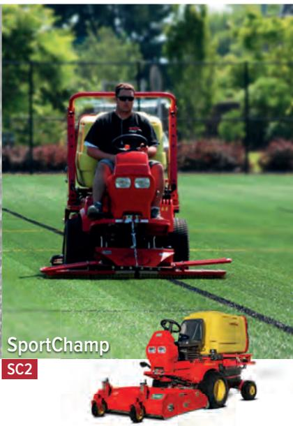
Multifunctional ride-on machine for the advanced maintenance of artificial turf.
