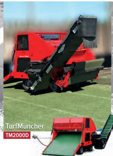
Self-propelled machine for the removal of artificial turf.
