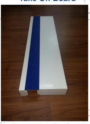
**40140:** The take-off board is made from hardened synthetic material. Its overall dimensions are 122x34x10 cm. The board consists of two sections of synthetic material. This item also includes an inlay board (40100), which is made from rubber and aluminium. The item is certified by the IAAF.
