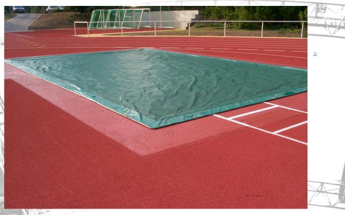
40180: The long jump sand pit cover is made from PVC coated netting fibre. The used material is spike proof. The cover is surrounded by a steel link chain. The cover weighs roughly 400 g/m<sup>2</sup>. The items are manufactured exactly in the size of the sand pit for an optimum coverage.
