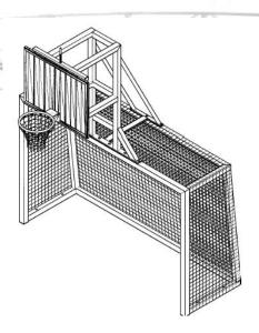
119626: Hobby Soccer Goal Post (3 x 2 m). "Open back with basketball attachment" Fully welded recreational goal made of high-grade aluminium profiles. The goal frame is made from our oval profiles (80 x 80 mm) with a wall thickness of 2.5 mm. Supplied with 4 ground anchors.
